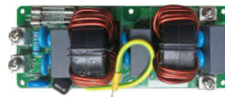
Filtering PCB (for 1 phase)
